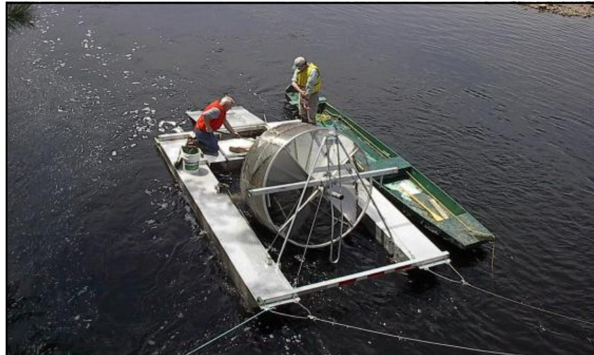
SMRA director Allan MacDonald and DFO biologist Peter Amiro tending the smolt wheel on the east branch of the St. Mary's River in May of 2003.
