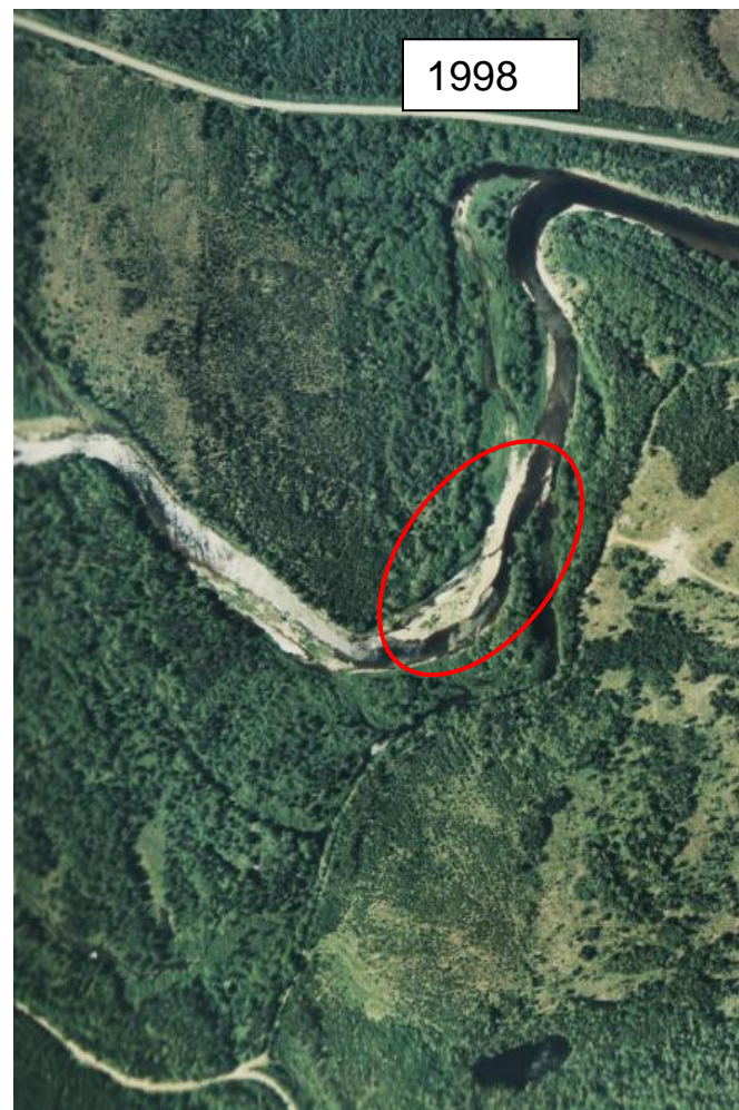
Plate 2: Air photographs of Section II at Sutherland's Brook confluence. Note lateral channel movement and braiding, as well as increased lateral bar formation (red ellipse).
