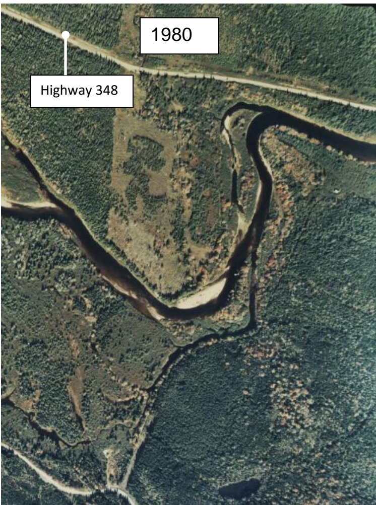
Plate 2: Air photographs of Section II at Sutherland's Brook confluence. Note lateral channel movement and braiding, as well as increased lateral bar formation (red ellipse).
