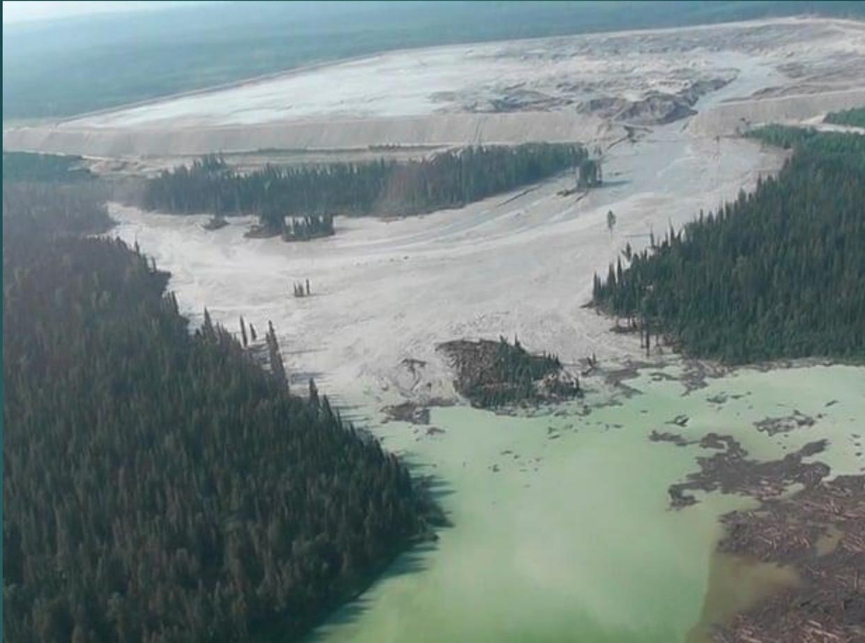
The results of a tailing pond breach at Imperial Metals Corp's gold and copper mine in Mount Polley BC in 2014, which released 24 million cubic meters of water and waste into the near by lakes and rivers which ultimately end up in the Fraser River. Photograph: Reuters
